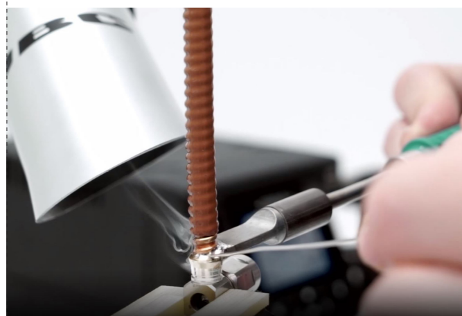
Soldering application using C470012 Cartridge
