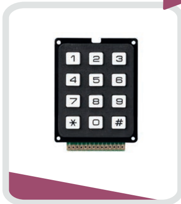
VEL 12KEY CLAVIER ALPHA- NUM 12 TOUCHES-SORTIE POINT COMMUN
