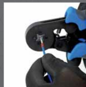
High-precision die geometry leads to a clearly defined crimp shape of the ferrule.
