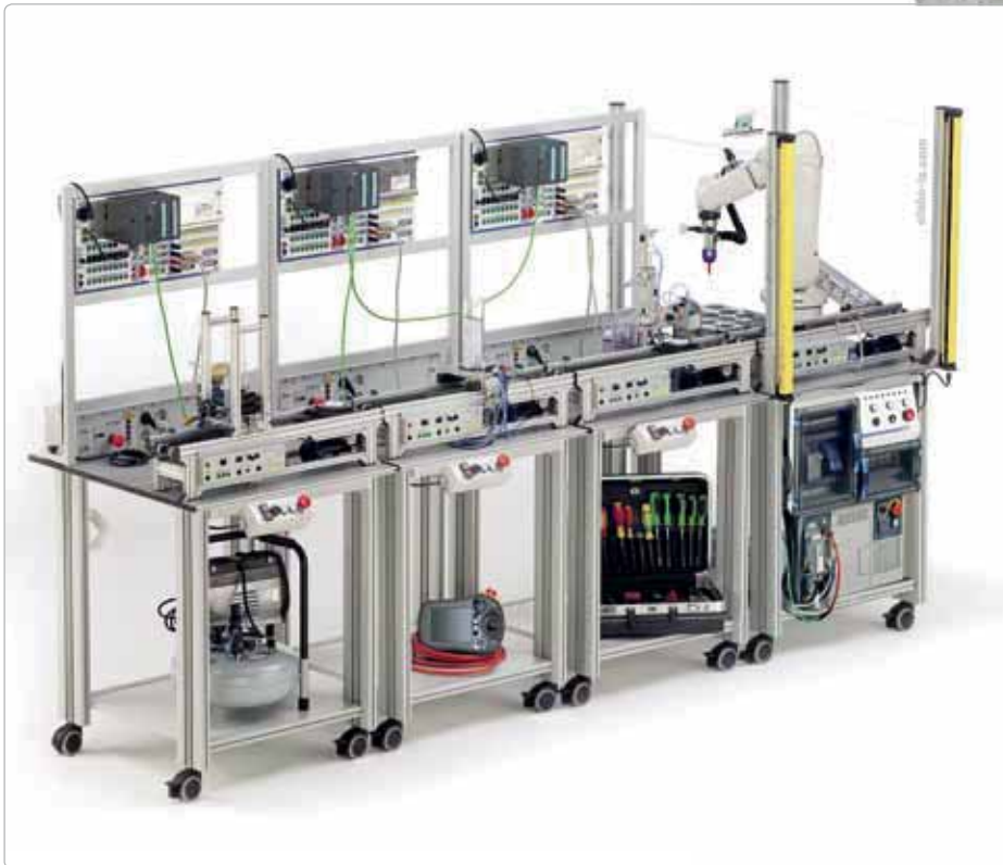
Modular production system with the robot cell SafetyCUBE®
